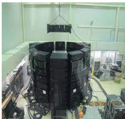
Example of DART setup for payload acoustic qualification (ref. NASASpaceFlight.com)
