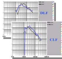
SEA-TEST reduces the subsystem FRF data and time decay data to a set of SEA parameters that completely describe how N&V energy will distribute itself in the test specimen. These parameters are effective mass (or acoustic volume), **Damping Loss Factor (DLF)**, **Coupling Loss Factor (CLF)**, modal density and power level of applied excitation.
